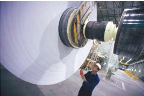
Finished reel of copy paper from the No5 machine
